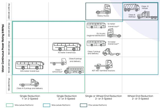
st 130kW motor variant planned for future release  $\,$  \*\* eIPA inverted portal axle - low floor applications
