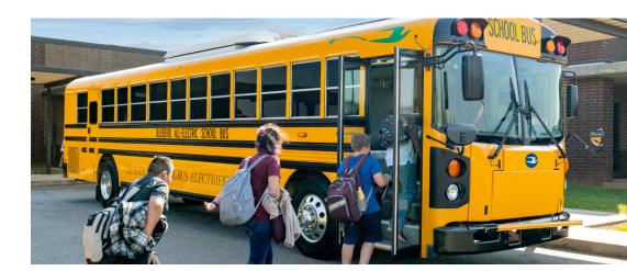
West Grand School District decided to add a <u>Blue Bird Type-D</u> <u>All-American electric bus</u> to their fleet in March of 2020. The bus features Accelera by Cummins PowerDrive 7000 system, which delivers high-efficiency and unmatched power, with module and flexible architecture, maintains existing mounting locations for easy OEM integration, delivers instant torque response, and has a lower total cost of ownership.
